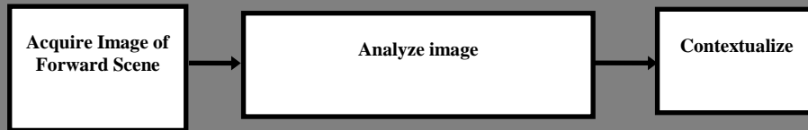
Figure 1: General block diagram of the image processing system
