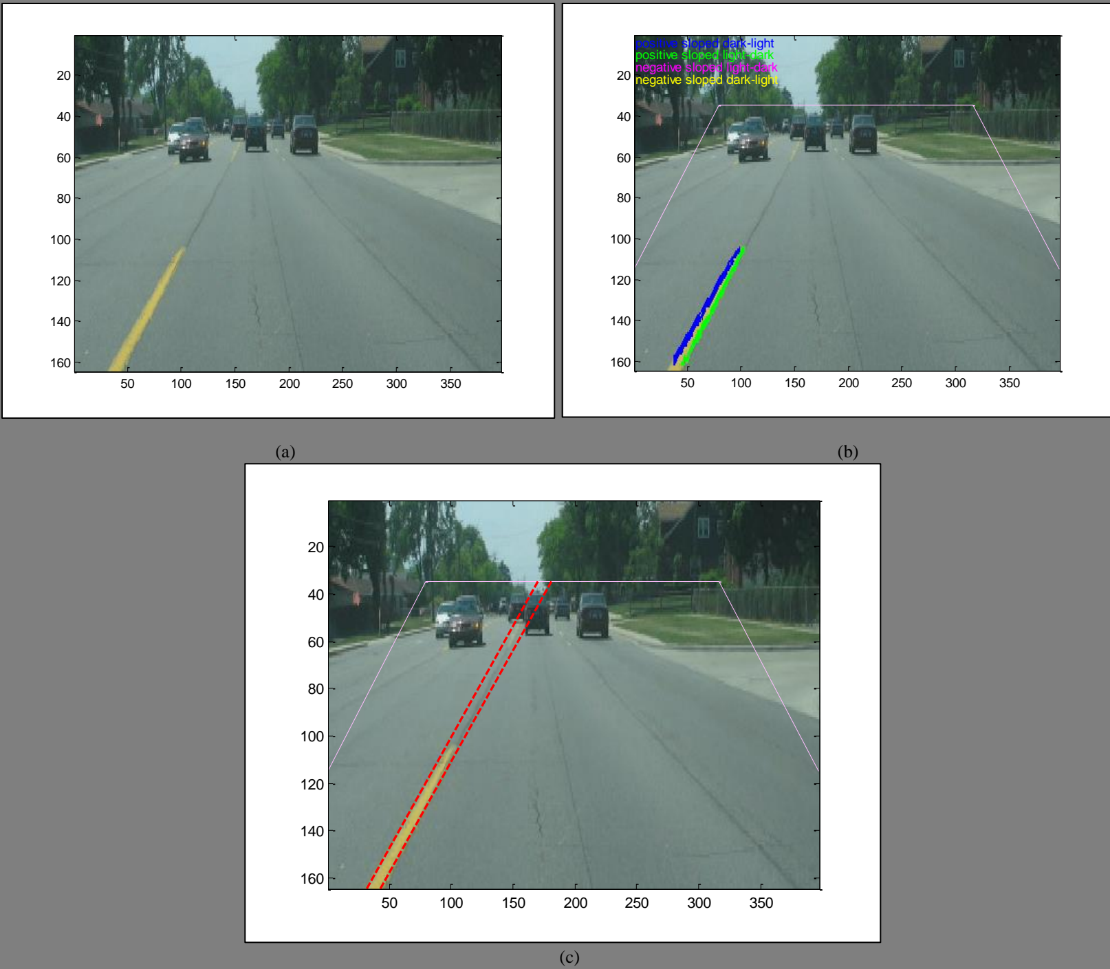
Figure X: (a) Cropped RGB image; (b) preliminary results of detection, connection, and GEM discrimination; (c) RGB cropped showing only positive sloped projections in red
